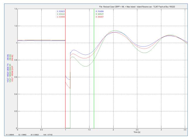
Figure 1 – Post-Fault Recovery Voltage Plot Three-Phase Fault at Sunnyside Terminal Station, resulting in a trip of TL267
