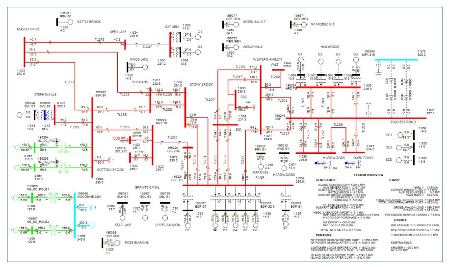
Figure 2 - Base Case 1 – Maximum Island Generation with 300 MW ML Import
